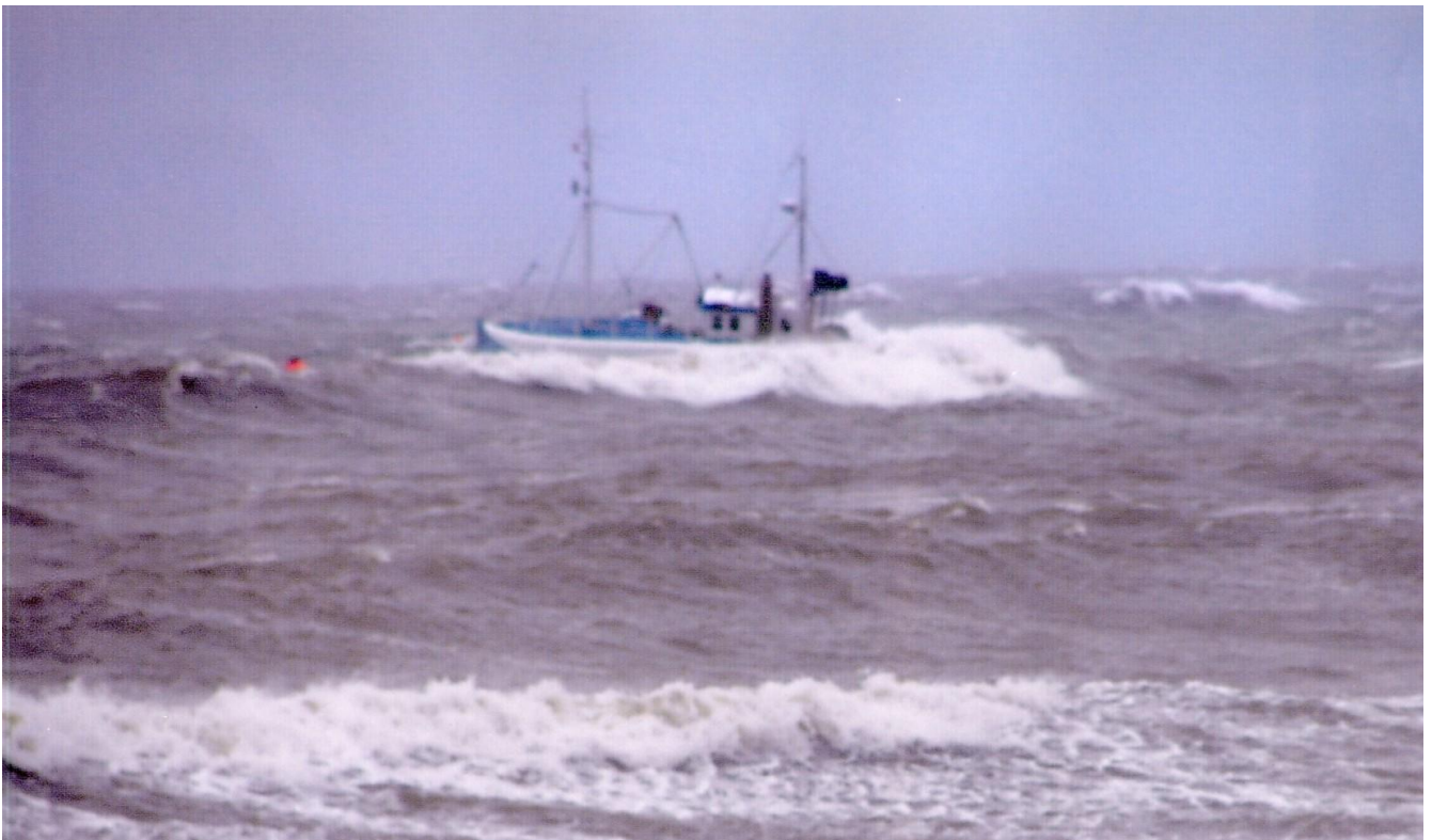
The fishers from Thorupstrand are using either cod gillnets with large meshes or Danish seine, which demands little energy and does not harness the sea floor and habitat. At the pictures a seaboat from Thorupstrand is hauling his Danish seine. Photo: Jan Olsen 2005.
